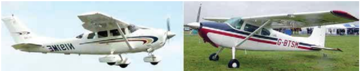
Figure 3 Nose Gear v. Tail Gear
