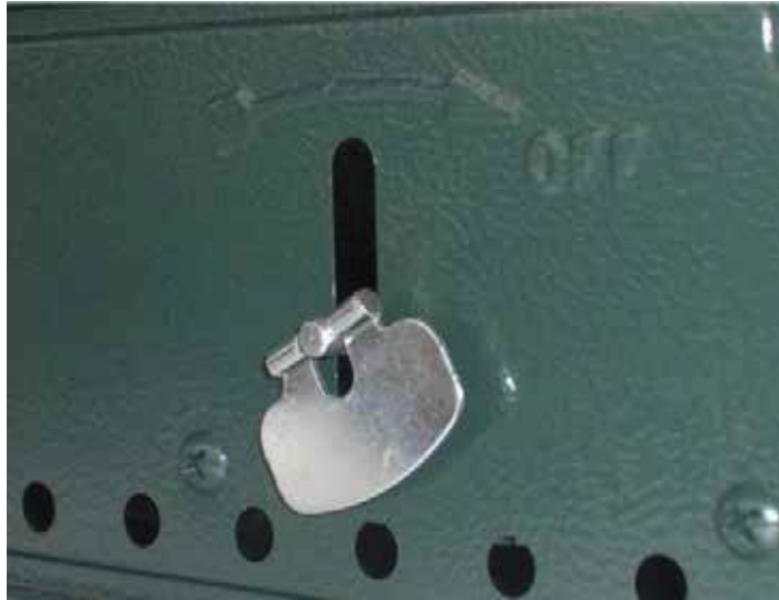
Figure 8 Auxiliary Burner Control
