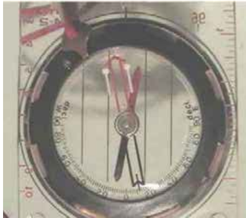
Figure 5 Declination Scale and Screw
