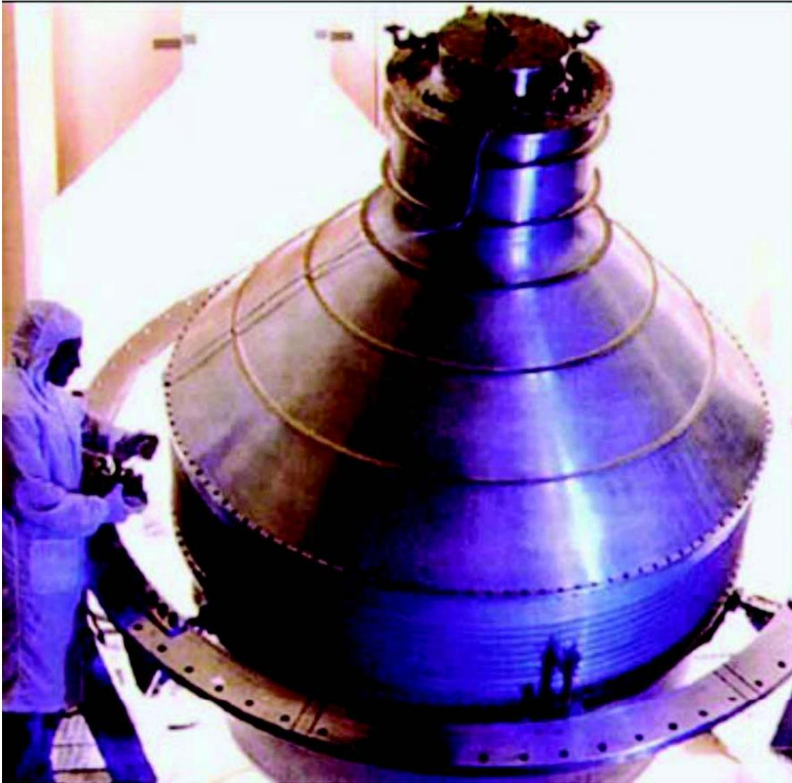
Figure A-2 Gravity Probe B Dewar
