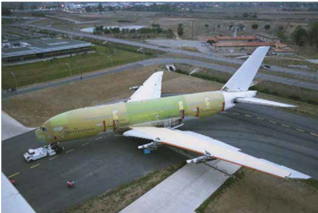
Figure B-4 Empty Pylons
