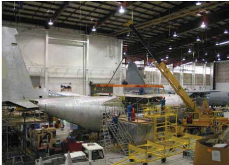
Figure A-2 Placing a C-130 Centre Wing
