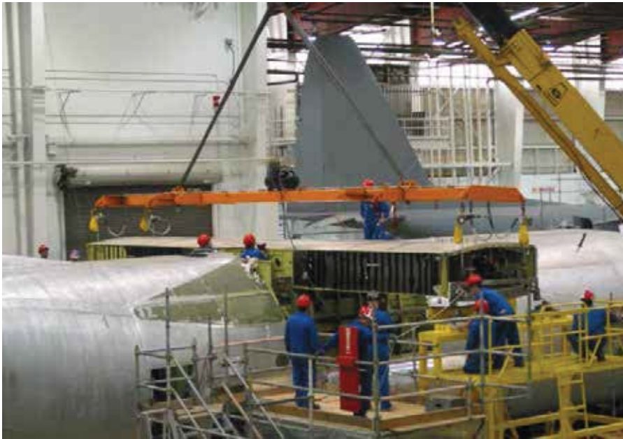
Figure A-3 Positioning a C-130 Centre Wing
