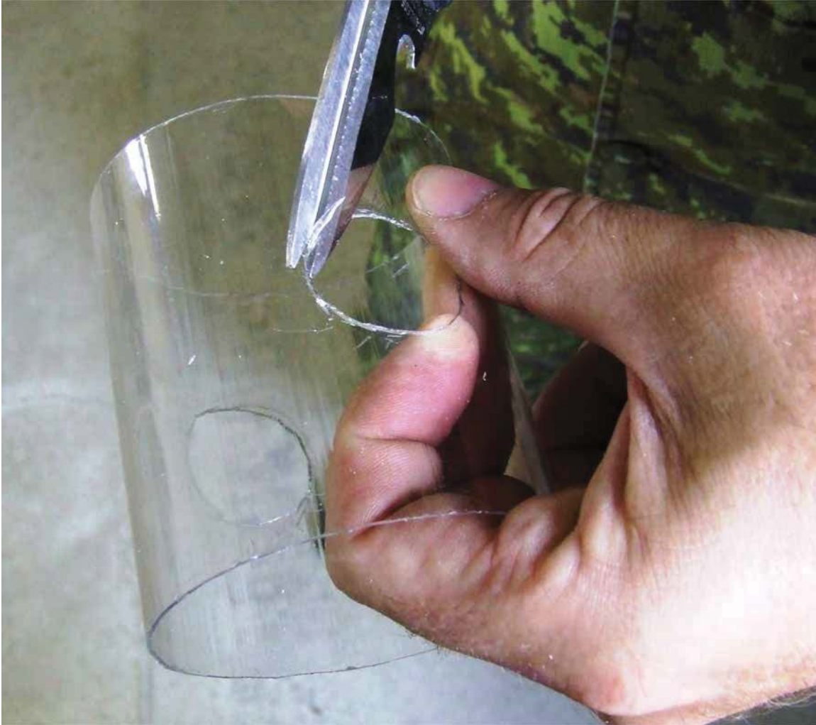
Figure 27-A Cutting the Hole in the Plastic Spring for Section A
