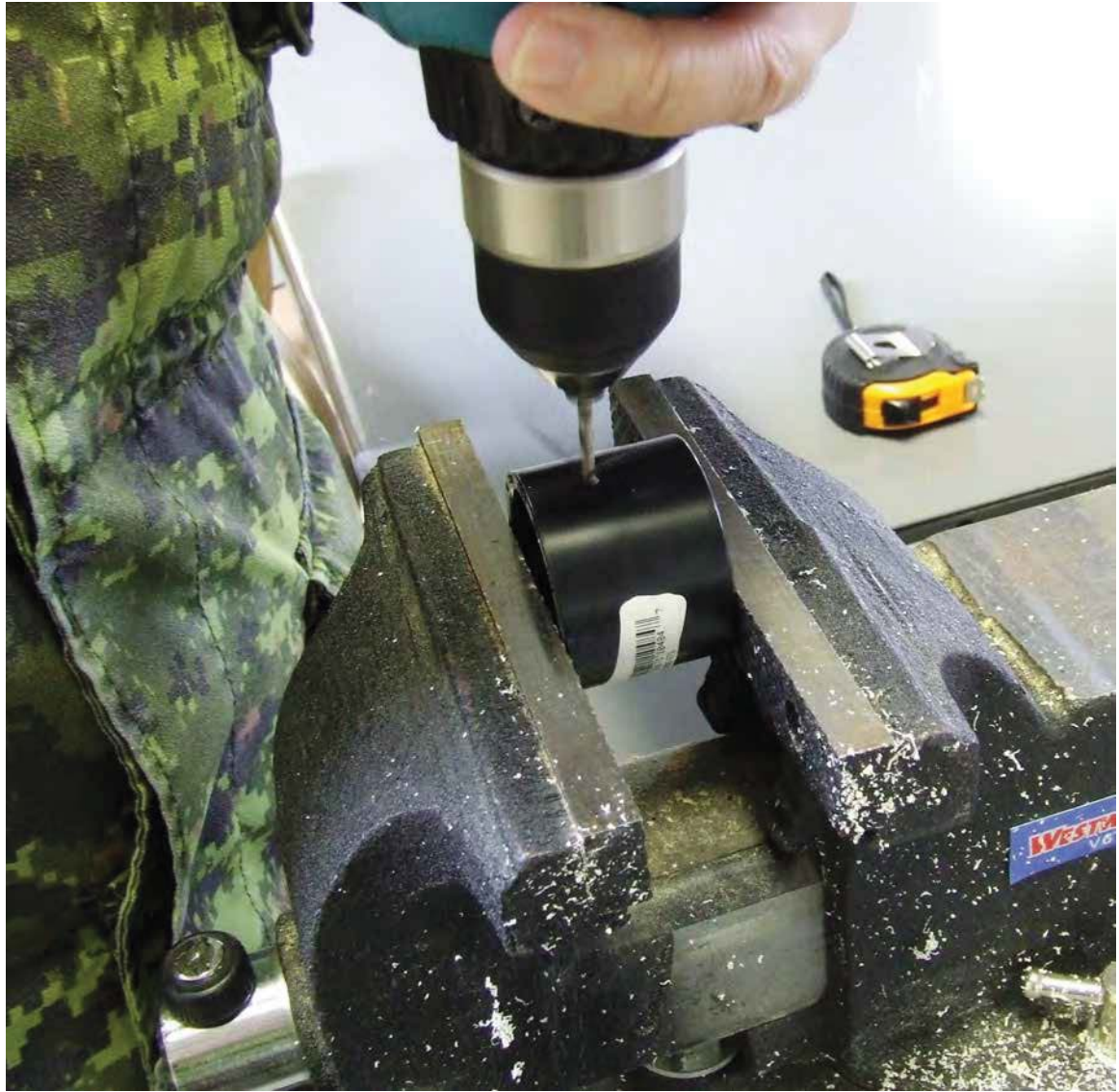
Figure 26-A Drilling 1/8-inch Holes in the ABS Coupler
