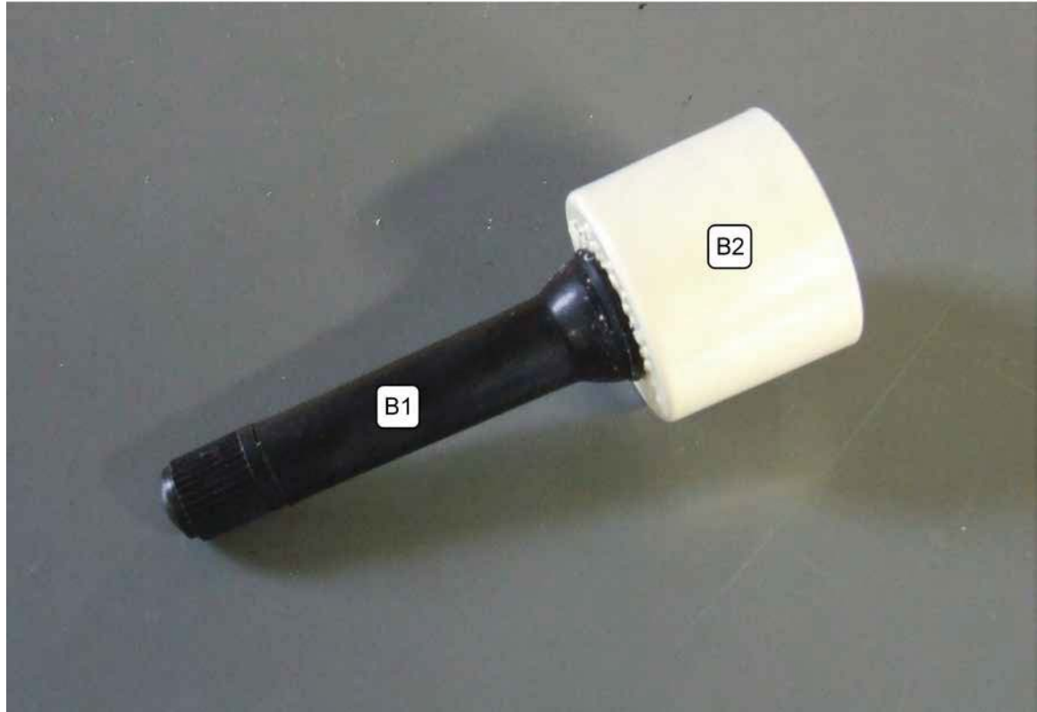
Figure 12-A Section B, Tire Valve Pulled Through B2
