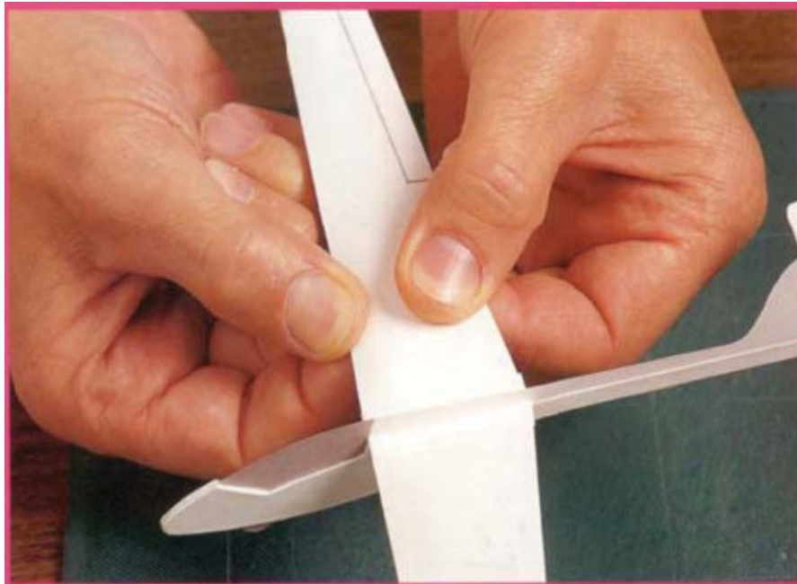
Figure 5 Adjusting Wing Curvature (Camber)
