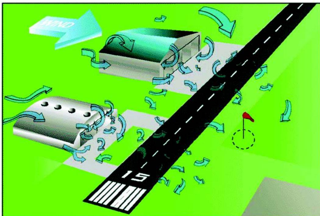
Figure 6 Mechanical Turbulence
