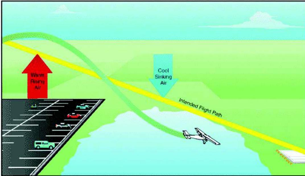
Figure 7 Thermal Turbulence
