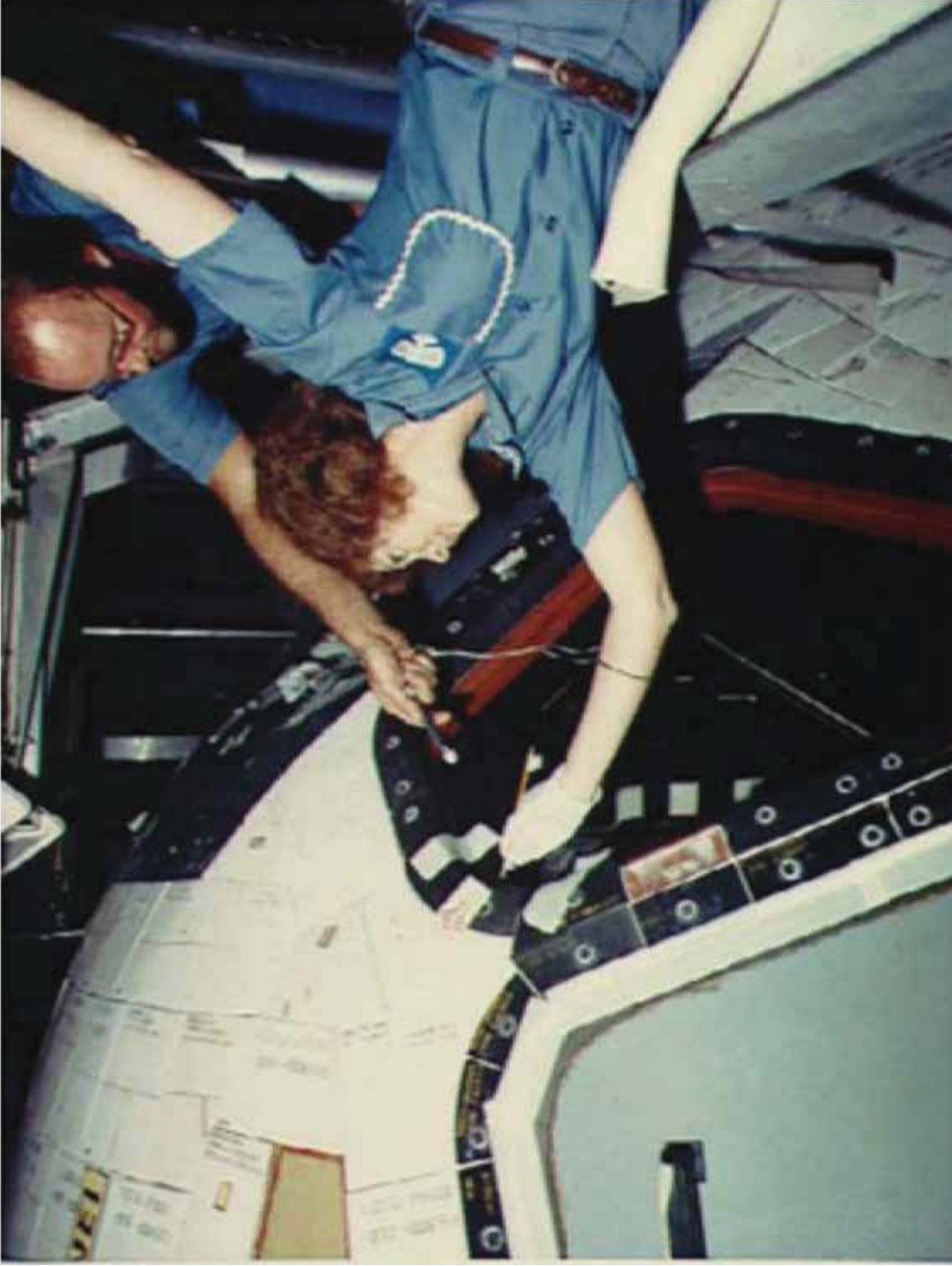
Figure B-3 Repairing TPS on Columbia
