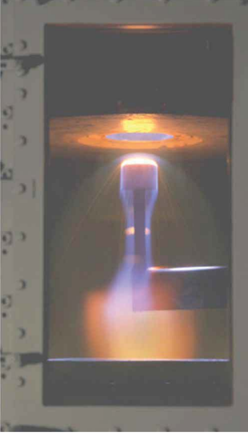
Figure B-1 Testing Thermal Insulation in a Wind Tunnel
